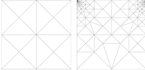
Figure 4: Initial (left, 16 elements) and adapted (right, 936 elements) meshes for the cavity problem ( $k = 1$ ).
