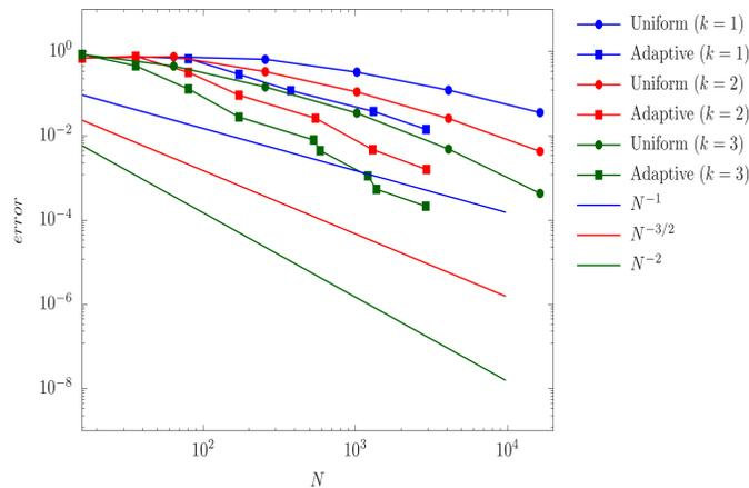
Figure 2: History of convergence for  $\mathbf{e}_h$  with uniform and adaptive ( $\theta = 0.25$ ) refinement ( $k = 1, 2, 3$ ), singularly perturbed problem.
