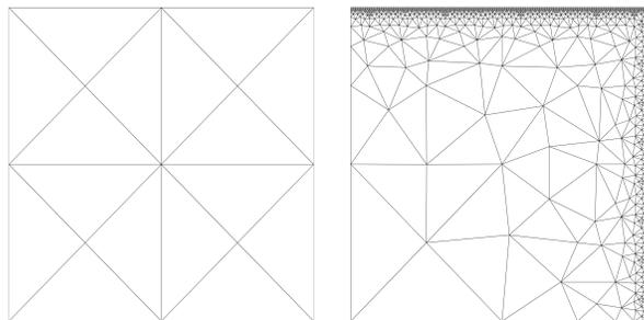
Figure 3: Initial (left, 16 elements) and final adapted (right, 2920 elements) meshes for the the singularly perturbed problem ( $k = 1$ ).
