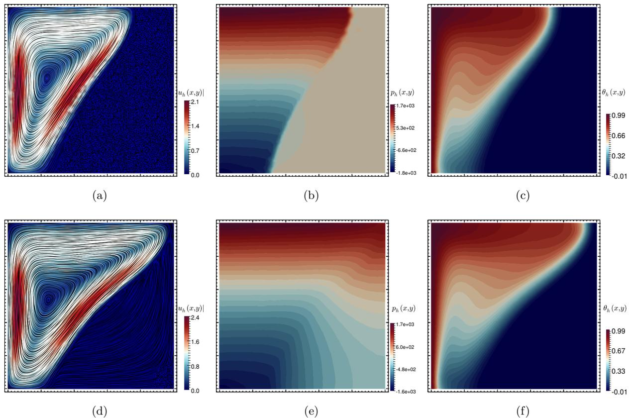
Figure 6.1: Example 3. Comparison between the melting of N-octadecane using enthalpy-viscosity (a,b,c) and enthalpy-porosity models (d,e,f).
