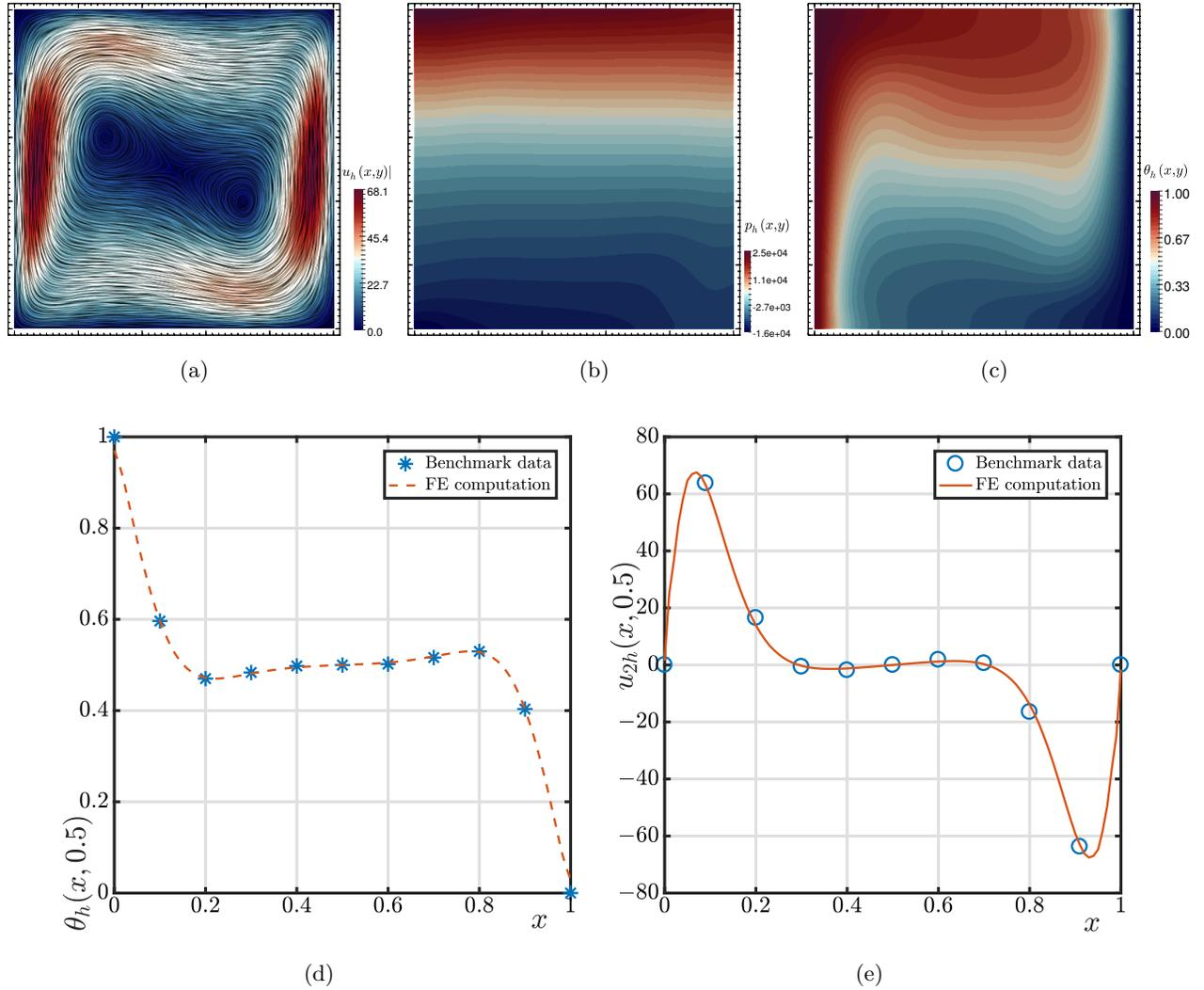
Figure 5.1: Velocity, pressure, and temperature profiles for the 2D differentially heated cavity (a,b,c respectively) and comparisons to the benchmark data in [48] (d and e).
