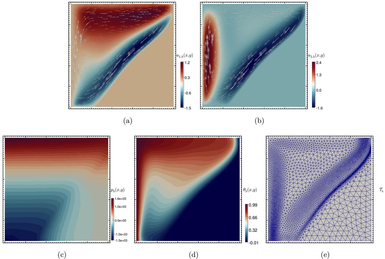
Figure 6.3: Example 4. Velocity components, pressure, temperature, and adapted mesh at  $t = 160$ , using a porosity-viscosity model with  $n = 5$ .
