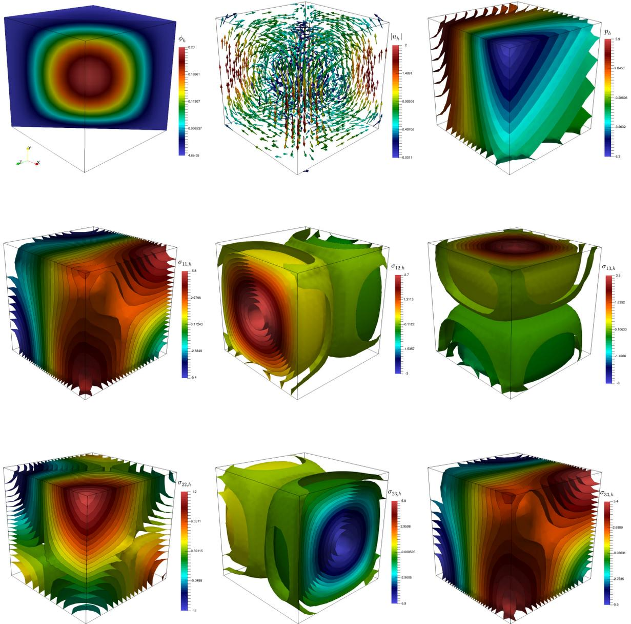
Figure 6.3: Numerical results for Example 3: From left to right and from up to down: approximation of scalar field concentration  $\phi_h$ , magnitude of the velocity  $\mathbf{u}_h$ , post-processed pressure  $p_h$ , and stress components. Snapshot obtained with 230705 DOF.
