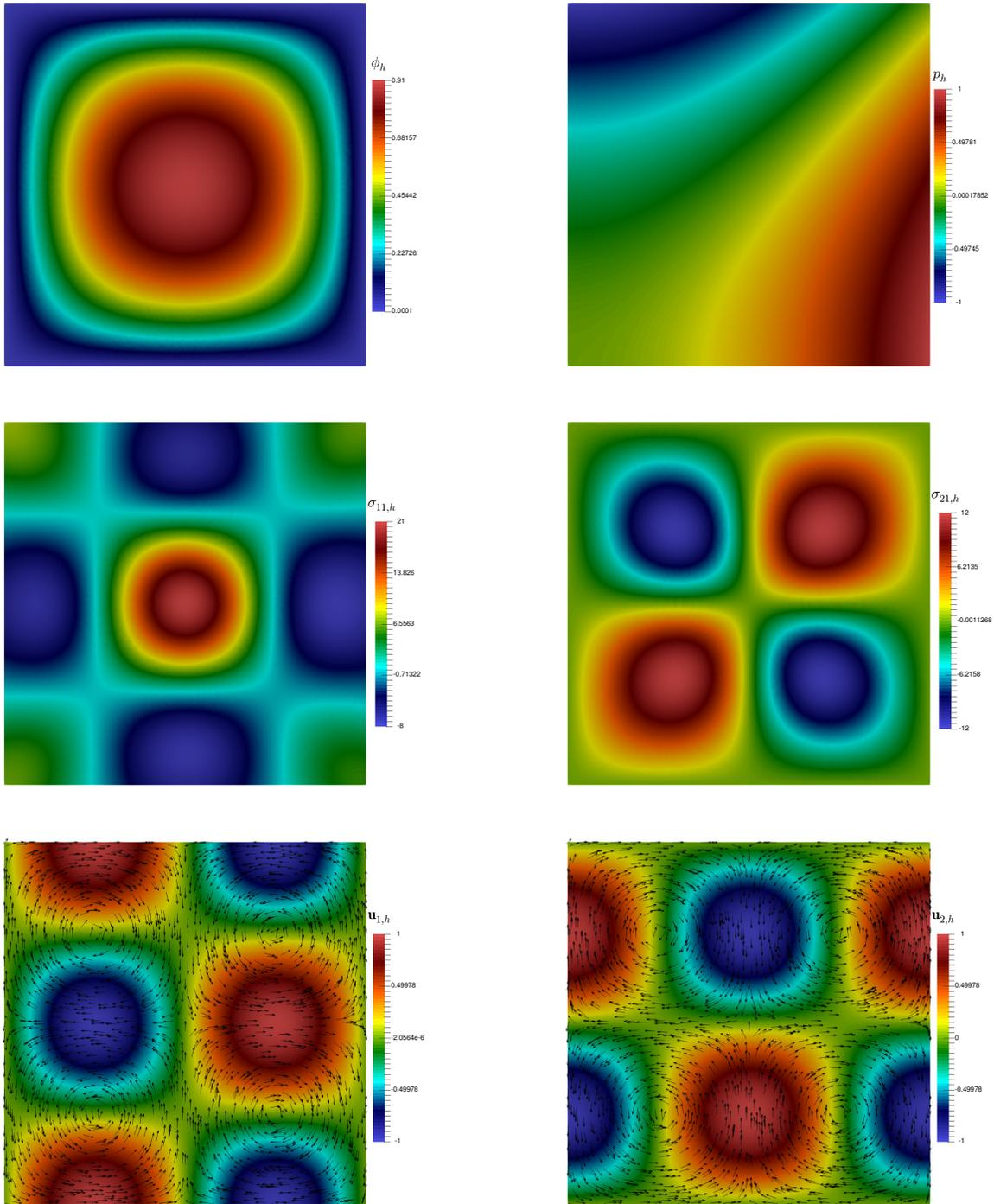
Figure 6.1: Numerical results for Example 1: From left to right and from up to down: approximation of scalar field concentration  $\phi_h$ , post-processed pressure  $p_h$ , stress and velocity components. Snapshot obtained from a simulation with 706165 DOF.
