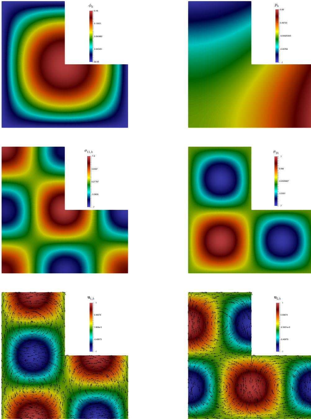
Figure 6.2: Numerical results for Example 2: From left to right and from up to down: approximation of scalar field concentration  $\phi_h$ , post-processed pressure  $p_h$ , stress components and velocity components. Snapshot obtained from a simulation with 498985 DOF.
