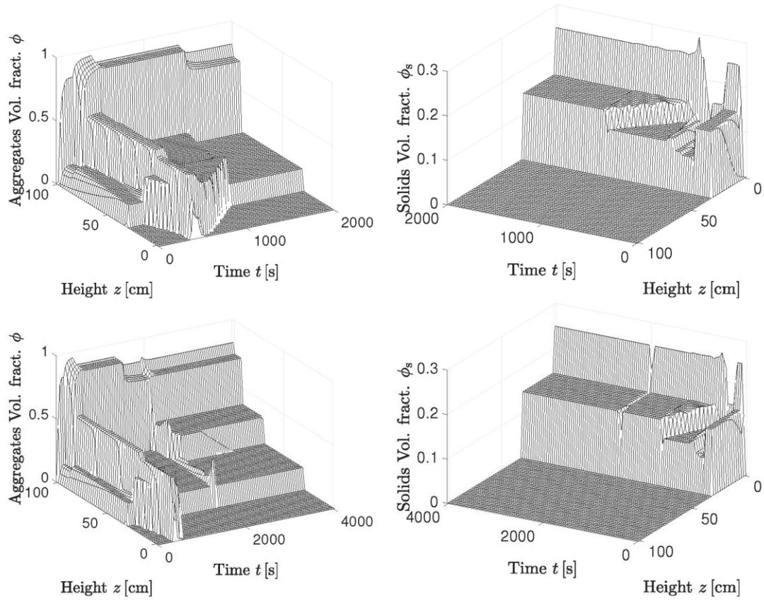
**Figure 4** Simulation of a flotation column with volume fractions of aggregates (left) and solids (right) as functions of height  $z$  [cm] and time  $t$  [s]. The upper row show the first 2000 seconds and the lower row the entire simulation to  $t = 4000$  s.
