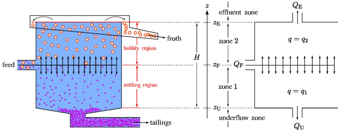
**Figure 2** Schematic of a DAF thickener (cf. Wang *et al.*, 2007) with constant cross-sectional area  $A = \pi 2.5^2 \text{ m}^2 = 19.635 \text{ m}^2$ , height  $H = 2 \text{ m}$  and feed inlet at  $z_F = 1 \text{ m}$ .
