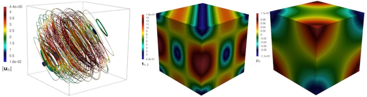
Figure 5.1: Example 1: velocity magnitude  $|\mathbf{u}_h|$ , concentration  $\phi_h$  and pressure  $p_h$  (left, center and right, respectively) obtained with the mixed-primal  $\mathbf{P}_0 - \mathbb{P}_0 - \mathbb{RT}_0 - \mathbf{P}_1$  approximation of a Brinkman flow with nonlinear transport using  $k = 0$  and  $N = 213,849$  degrees of freedom.
