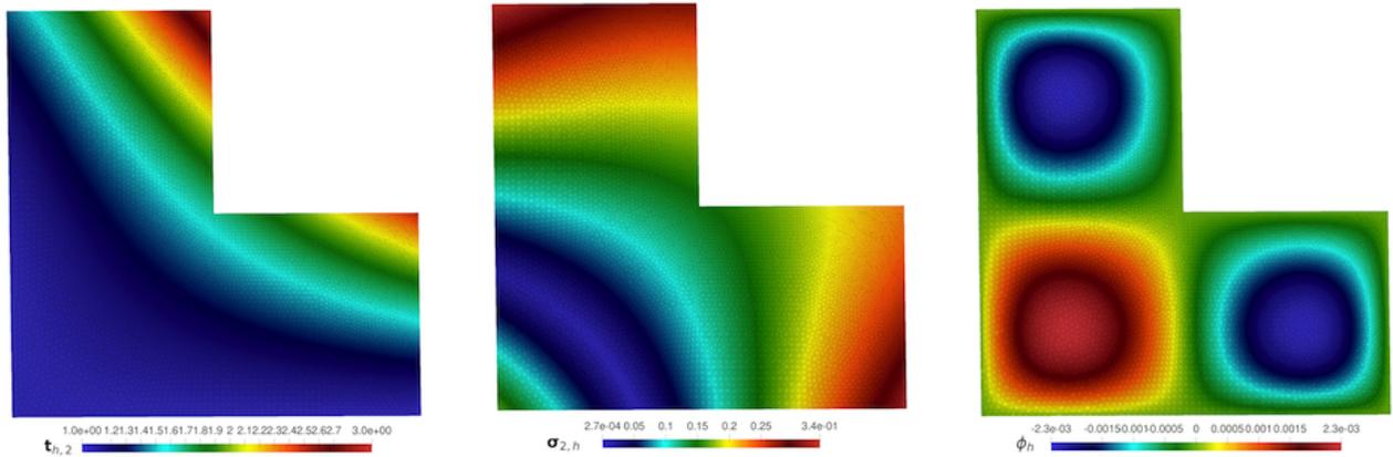
Figure 5.2: Example 2: components  $\mathbf{t}_{h,2}$  and  $\boldsymbol{\sigma}_{h,2}$  of the velocity gradient and the tensor  $\boldsymbol{\sigma}_h$  (left and center, respectively) and pressure  $p_h$  obtained with the mixed-primal method for a Brinkman flow with nonlinear transport using  $k = 1$  and  $N = 291,691$  degrees of freedom.
