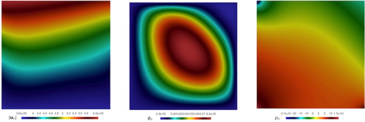
Figure 5.3: Example 3: velocity magnitude  $|\mathbf{u}_h|$ , concentration  $\phi_h$  and pressure  $p_h$  (left, center and right, respectively) obtained with the mixed-primal method of a Brinkman flow problem with nonlinear transport and no manufactured analytical solution using  $k = 0$  and  $N = 213,849$  degrees of freedom.
