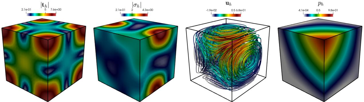
Figure 5.3: Sample of approximate solutions (velocity with streamlines) for the convergence test, obtained using the first-order PEERS-based finite element family.
