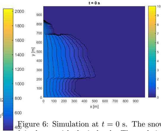
Figure 6: Simulation at  $t = 0$  s. The snow depth  $h$  is shown with the isolevels. The scale is in m.
