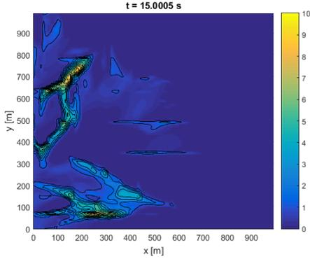
Figure 9: Simulation at  $t = 15$  s. The snow depth  $h$  is shown with the isolevels. The scale is in m.
