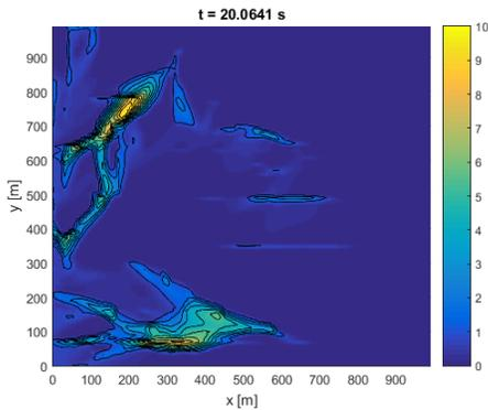
Figure 10: Simulation at  $t = 20$  s. The snow depth  $h$  is shown with the isolevels. The scale is in m.
