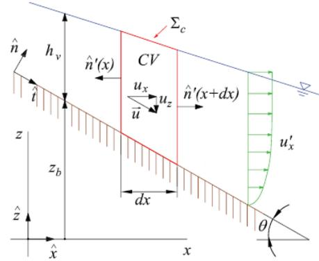
Figure 1: Control volume ( $x$  is horizontal axis and  $z$  is vertical axis).  $h_v$  is the height of the fluid,  $z_b$  is the height of the terrain topography and  $u_x$  is the velocity component in  $x$ .
