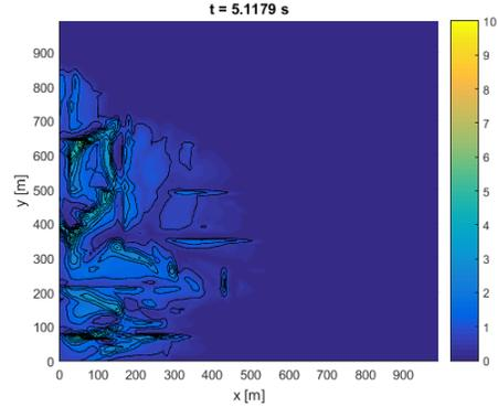
Figure 7: Simulation at  $t = 5$  s. The snow depth  $h$  is shown with the isolevels. The scale is in m.
