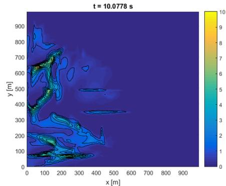
Figure 8: Simulation at  $t = 10$  s. The snow depth  $h$  is shown with the isolevels. The scale is in m.
