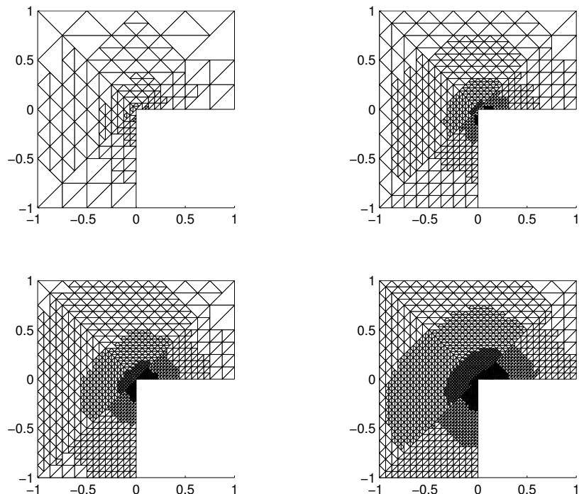
**Figure 5.6.16:** Example 3 with  $\mathbf{P}_0 - \mathbf{P}_0 - \mathbf{P}_1 - \mathbf{P}_0$  approximation, with hanging nodes: adapted intermediate meshes with 3661, 13111, 25531 and 48616 degrees of freedom.
