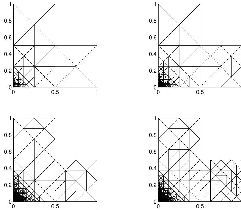
**Figure 5.6.11:** Example 2 with  $\mathbf{P}_1 - \mathbf{P}_1 - \mathbf{P}_2 - \mathbf{P}_1$  approximation, without hanging nodes: adapted intermediate meshes with 5305, 16732, 41692 and 62323 degrees of freedom.
