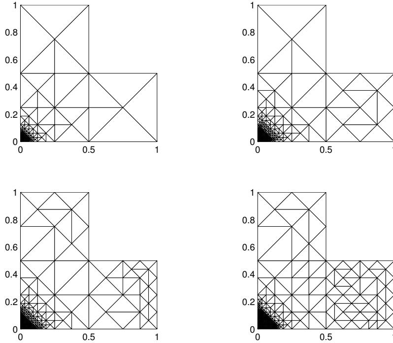
**Figure 5.6.9:** Example 2 with  $\mathbf{P}_0 - \mathbf{P}_0 - \mathbf{P}_1 - \mathbf{P}_0$  approximation, without hanging nodes: adapted intermediate meshes with 5011, 13636, 22321 and 52306 degrees of freedom.
