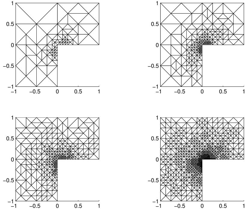
**Figure 5.6.17:** Example 3 with  $\mathbf{P}_1 - \mathbf{P}_1 - \mathbf{P}_2 - \mathbf{P}_1$  approximation, without hanging nodes: adapted intermediate meshes with 4954, 12676, 20097 and 49453 degrees of freedom.
