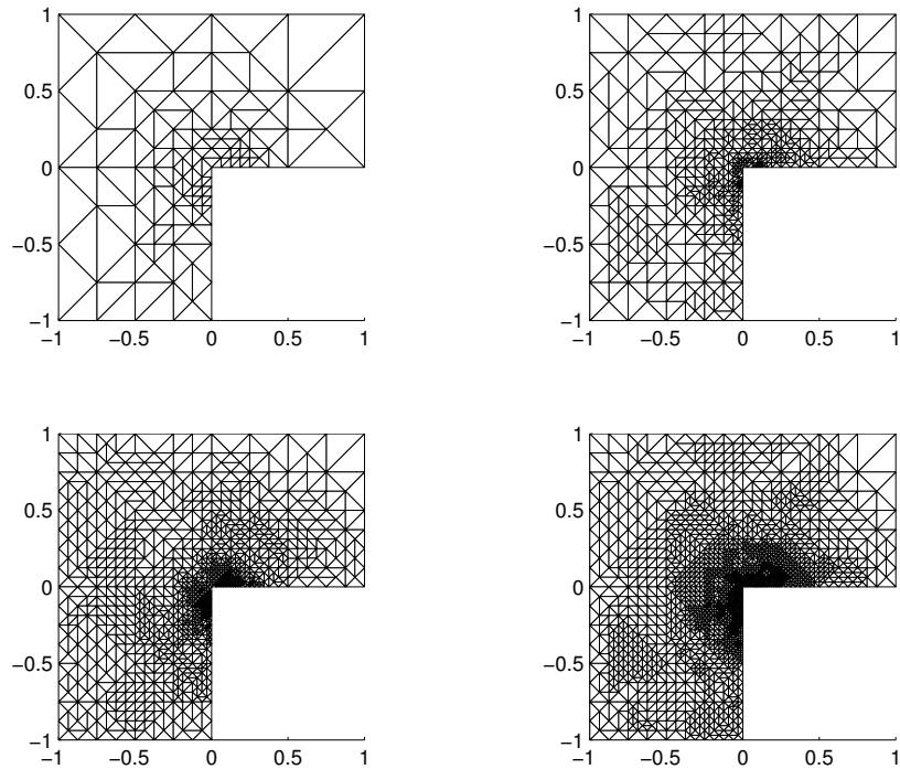
**Figure 5.6.15:** Example 3 with  $\mathbf{P}_0 - \mathbf{P}_0 - \mathbf{P}_1 - \mathbf{P}_0$  approximation, without hanging nodes: adapted intermediate meshes with 2566, 12256, 26416 and 48766 degrees of freedom.
