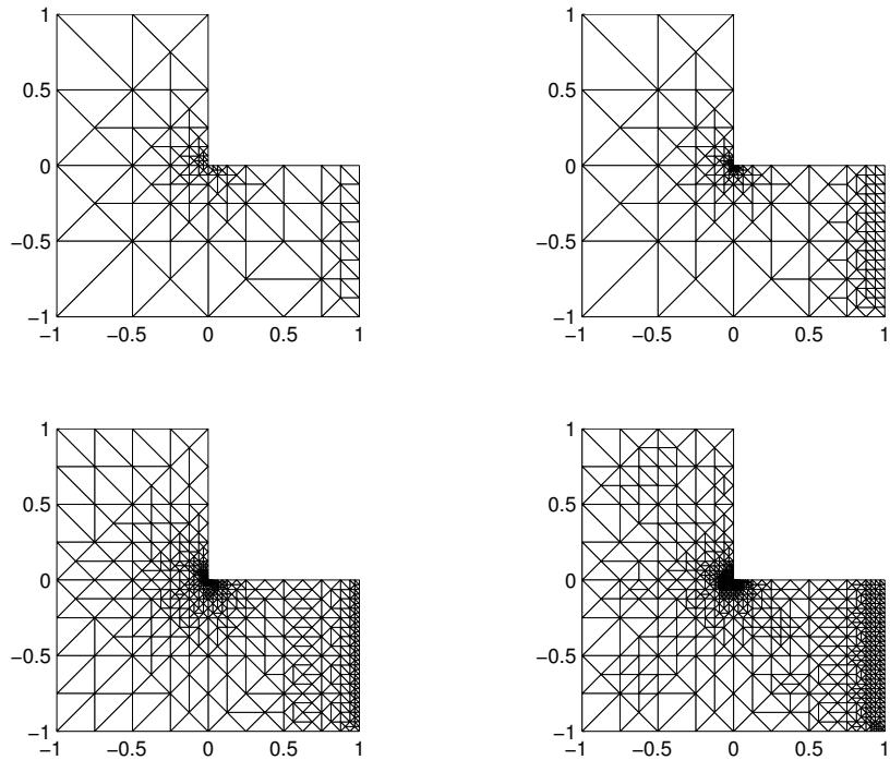
**Figure 5.6.23:** Example 4 with  $\mathbf{P}_1 - \mathbf{P}_1 - \mathbf{P}_2 - \mathbf{P}_1$  approximation, without hanging nodes: adapted intermediate meshes with 6826, 12910, 35608 and 55420 degrees of freedom.
