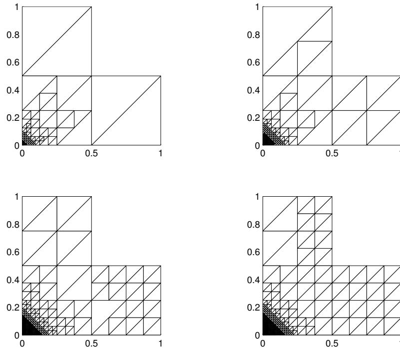
**Figure 5.6.12:** Example 2 with  $\mathbf{P}_1 - \mathbf{P}_1 - \mathbf{P}_2 - \mathbf{P}_1$  approximation, with hanging nodes: adapted intermediate meshes with 4681, 12988, 32878 and 51247 degrees of freedom.
