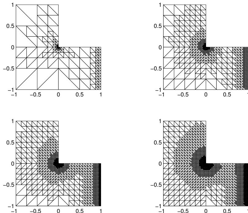
**Figure 5.6.22:** Example 4 with  $\mathbf{P}_0 - \mathbf{P}_0 - \mathbf{P}_1 - \mathbf{P}_0$  approximation, with hanging nodes: adapted intermediate meshes with 3781, 16741, 31411 and 57376 degrees of freedom.
