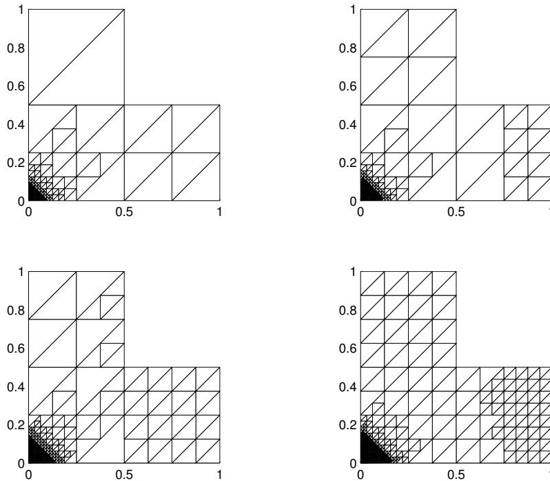
**Figure 5.6.10:** Example 2 with  $\mathbf{P}_0 - \mathbf{P}_0 - \mathbf{P}_1 - \mathbf{P}_0$  approximation, with hanging nodes: adapted intermediate meshes with 6841, 14941, 30826 and 64801 degrees of freedom.
