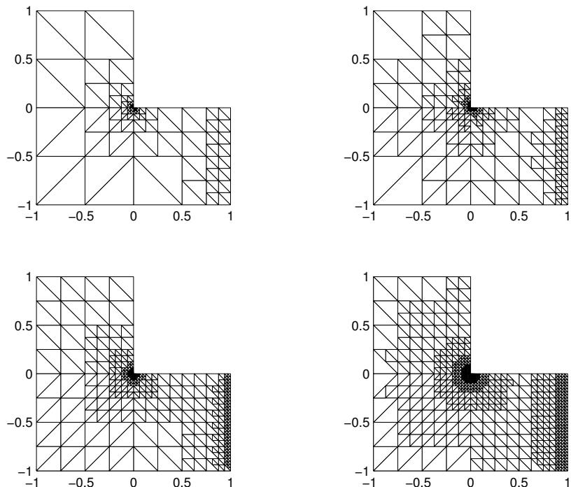
**Figure 5.6.24:** Example 4 with  $\mathbf{P}_1 - \mathbf{P}_1 - \mathbf{P}_2 - \mathbf{P}_1$  approximation, with hanging nodes: adapted intermediate meshes with 5617, 14041, 23635 and 49843 degrees of freedom.
