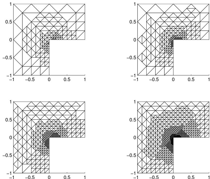
**Figure 5.6.18:** Example 3 with  $\mathbf{P}_1 - \mathbf{P}_1 - \mathbf{P}_2 - \mathbf{P}_1$  approximation, with hanging nodes: adapted intermediate meshes with 8113, 12793, 20398 and 43447 degrees of freedom.
