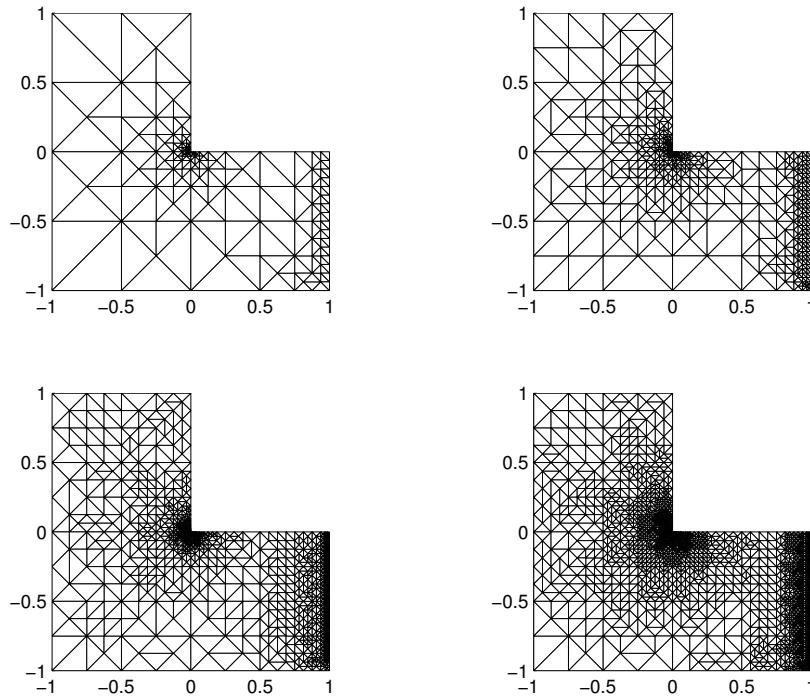
**Figure 5.6.21:** Example 4 with  $\mathbf{P}_0 - \mathbf{P}_0 - \mathbf{P}_1 - \mathbf{P}_0$  approximation, without hanging nodes: adapted intermediate meshes with 3946, 14311, 30286 and 58306 degrees of freedom.
