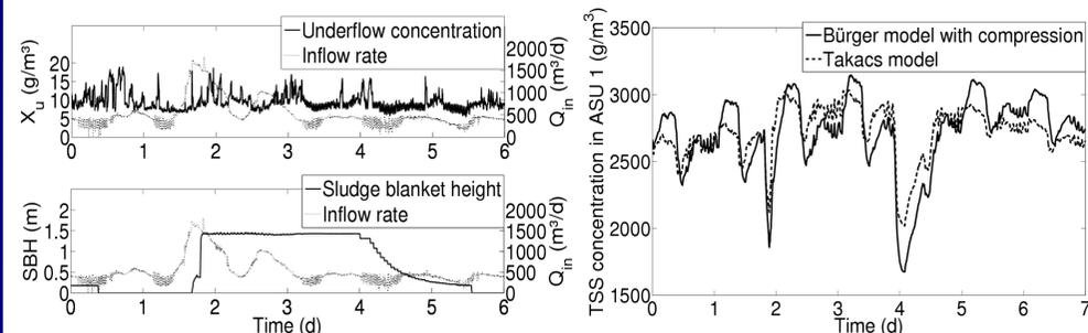
**Figure 2:** On-line data of sludge blanket height (SBH), underflow concentration ( $X_u$ ) and inflow rate ( $Q_{in}$ ) from the WWTP of Eindhoven, The Netherlands (left) and dynamic simulation results of the BSM1 MLSS concentration in ASU1 (right).
