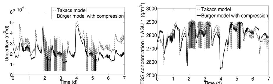
**Figure 3:** Dynamic simulation with the implementation of an MLSS control strategy. Manipulation in underflow rate (left) and MLSS concentration in the first activated sludge tank (right) under storm weather conditions.
