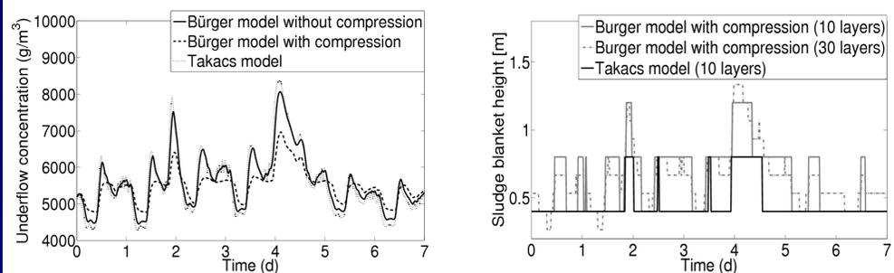
**Figure 1:** Dynamic simulation of the underflow concentration (left) and the sludge blanket height (right) under storm weather conditions.
